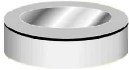
Glue the completed filter cell onto the cylinder to complete construction.
